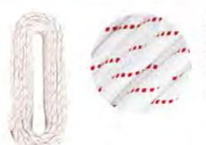
Excellent static rope designed for technical use for rope access, rescue and for manipulation with the objects. Meet NFPA 1983 Technical Use requirements that the rescuers, firemen, specialists working at height and other professionals require when working every day. Weight: 72 g/m • Strength: 32 kN Length: pack: 150, 200, 300 ft / 46, 61, 92 m spool: 330, 600, 660 ft / 100, 183, 200 m Diameter: 10.5 mm
