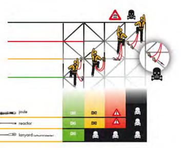
When safeguarding an ascent using a fall arrest type "Y" it is necessary to move at the level FF1 and lower. It means that the connectors (EN362) connected to the fall absorber (EN355) during the ascent do not "fall" below the connection point of the harness (EN361) in which the absorber is connected to the harness.
