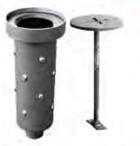
Flush floor sleeve with 3/8" drainage pipe connection to be installed to existing concrete by core-drilling and resin fix. A suitable shrink-free grout is PCI swelling mortar with the designation "Grout 100".
