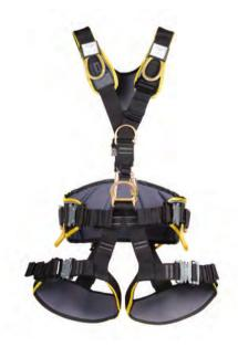
The variant of EXPERT 3D harness according to the North American standards ANSI and NFPA with SPEED buckles, metal elements made of steel, fall indicators and lanyard keepers.
