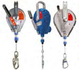
Self-retractable arrester with built in two-way rescue/ recovery mechanism. Fall arrest device with rescue lifting and lowering facility, equipped with a recovery mechanism operated by a device mounted handle. After an arrested fall, or if the user becomes incapacitated at the bottom of a shaft, the recovery mechanism can easily be engaged by a second person to raise or lower the person to a place of safety.
