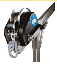
Hand crank winch for easy and jerk-free lifting and lowering of persons and loads according to Directive 2006/42/EG with 30 m stainless steel rope of Ø 6mm (min. breaking load 18.76 kN). SWL is 300 Kg. Material: stainless steel 1.4571 (V4A), PA Dimensions: 230 x 336 x 200 mm (length x width x height) Weight: 18,5 kg CE • EN 1808:2015
