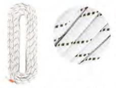
Excellent static rope, meet NFPA 1983 Technical Use requirements that the rescuers, firemen, specialists working at height and other professionals require when working every day. Manufactured by patented rope-braiding technology ROUTE 44 with ultrosonic ending. Weight: 77 g/m • Strength: 33.5 kN Length: pack: 150, 200, 300 ft / 46, 61, 92 m spool: 330, 600, 660 ft / 100, 183, 200 m Diameter: 11.0 mm • 7/16 in
