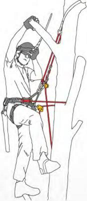
One of the most effective options of getting into the tree is setting up ascent ropes from the ground. It is done by throwing a light bag carrying a thin rope over the required anchor point. The ascent system is then pulled by this light rope. There are two common methods of climbing: Single Rope System (SRS) and Moving Rope System (MRS).
